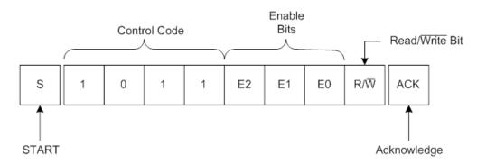
Upon receiving the correct Control Code, the chip enable bits, and the R/W bit, the device performs an acknowledge by pulling the SDA line low during the 9th clock pulse. As stated above, the device will now be set for either a read or a write operation by the R/W bit.
