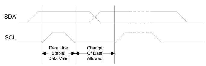
Figure 3-1. Bit Transfer on the I<sup>2</sup>C bus
